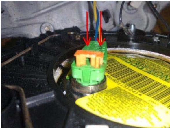
Get on the connector of the air-bag, green color
