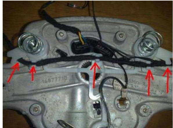
Clasp the cable of the paddles
