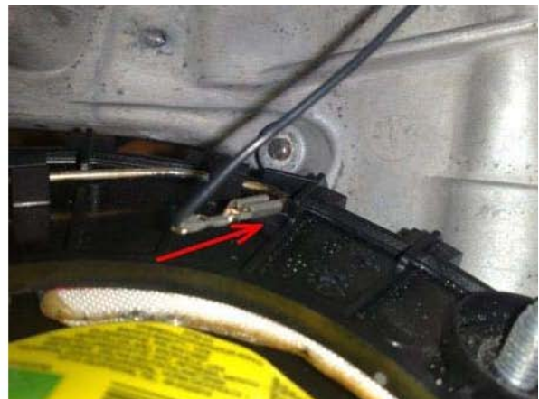
Get on the connector of horn
