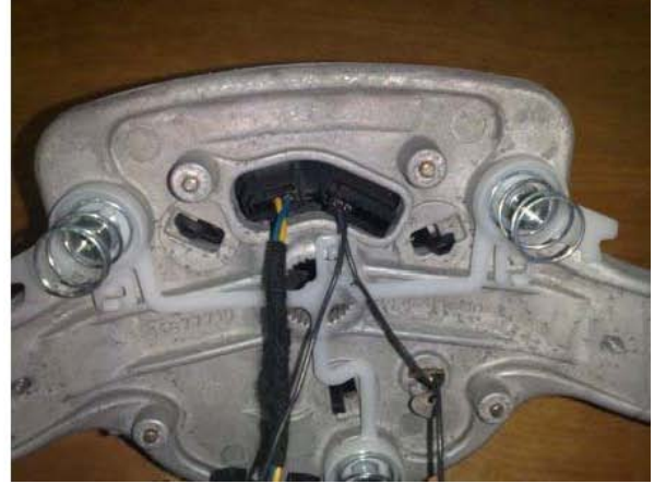
Unscrew the three screws (Torx 40) for get off the air-bag
