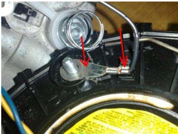
Get on the connector of horn
