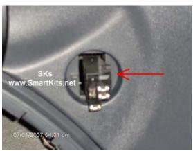
In the passenger door, unplug the window switch and pull out the connector
