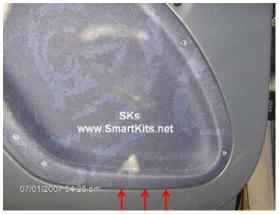
Pull the bottom of the door card away from the door, you will hear the clips coming undone. Side the door card forward to remove
