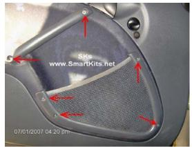
Remove the handle and the door pocket using Torx 20 and Torx 25 screwdrivers.
