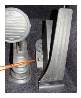
Loosen these 2 nuts attaching the accelerator pedal using a 13mm socket or wrench and lift out the pedal
