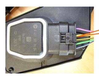
To undo the cable/plug there's a tab you have to press and then it pulls out.
