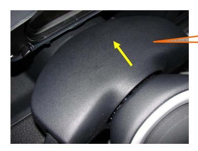
Remove this Cover (pull) on the upper side of the steering column cover
